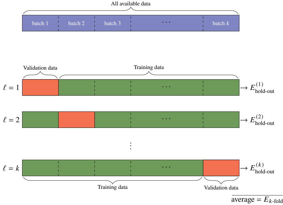
Figure 4.2: Illustration of k -fold cross-validation. The data is split into k batches of similar sizes. When looping over \ell = 1, 2, \dots, k , batch \ell is held out as validation data, and the model is trained on the remaining k - 1 data batches. Each time, the trained model is used to compute the average error E_{k\text{-fold}}^{(\ell)} for the validation data. The final model is trained using all available data, and the estimate of E_{\text{new}} for that model is E_{k\text{-fold}} , the average of all E_{k\text{-fold}}^{(\ell)} .
